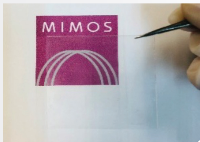
Coating showing low haze and high optical transparency
