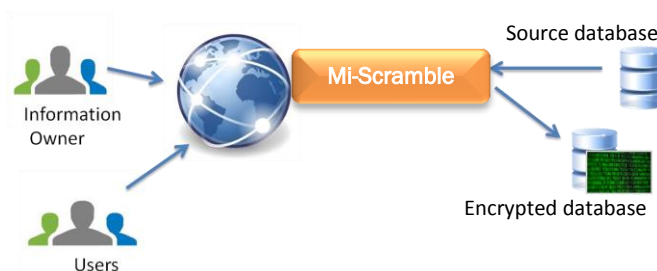
MIMOS Mi-Scramble system architecture
