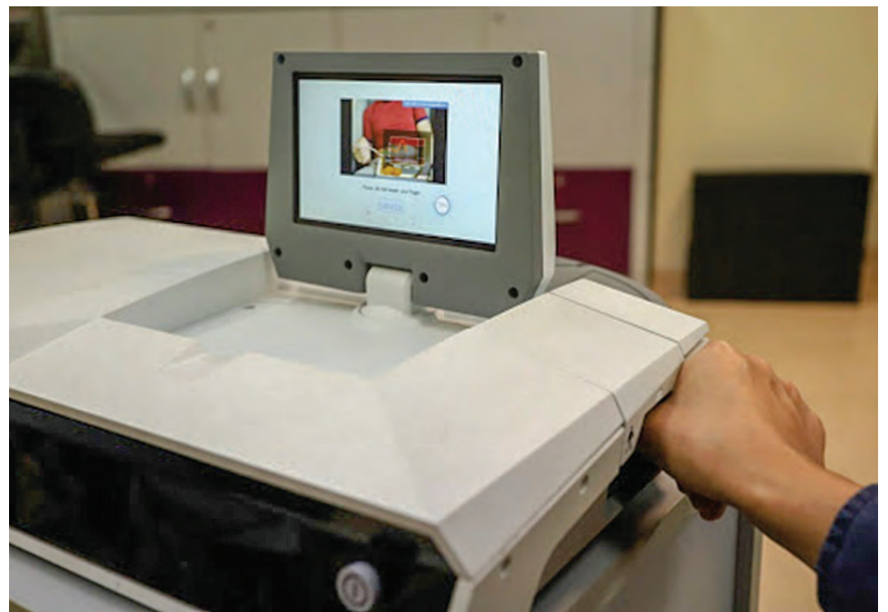
The GlucoSenz is a non-invasive blood glucose monitoring device.
